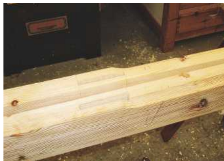
▲ Pic.6 The stopped rebates and grooves for the boards were also made at this point
